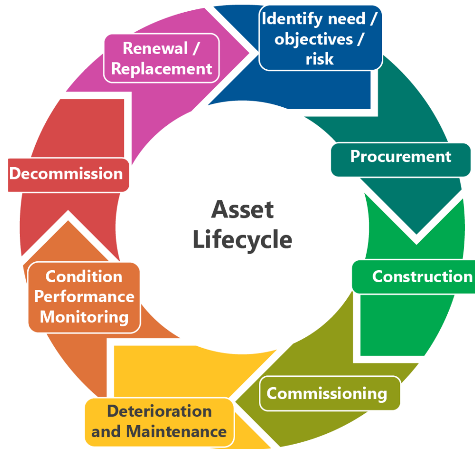
Figure 5-2: Asset Lifecycle Steps from Need Identification to Replacement
