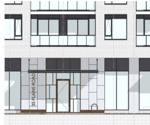
Partial East Elevation - Residential Entry
